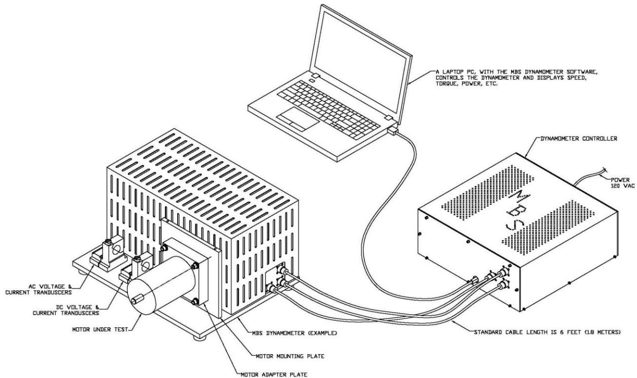
Dynamometers, or more specifically the size of the brakes for the dynamometers, are selected based on the required power dissipation and required torque.
